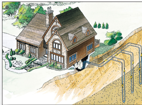
Example of a vertical, closed-loop system.
